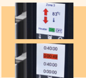
HDW-TTC Option Shown: Temperature adjustment and timer touchscreen control
